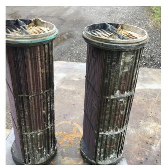
These after-coolers that were cleaned for a customer in the marine industry.
